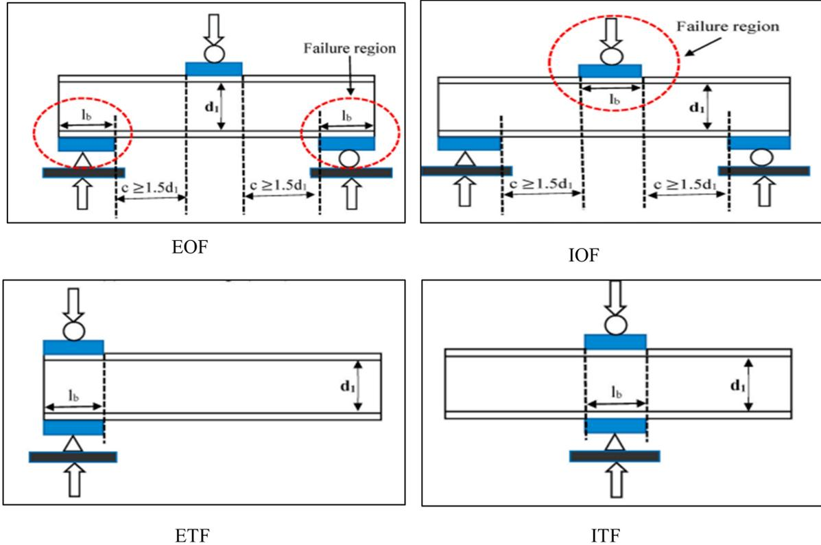
Figure 1: Web crippling failure types [2]
