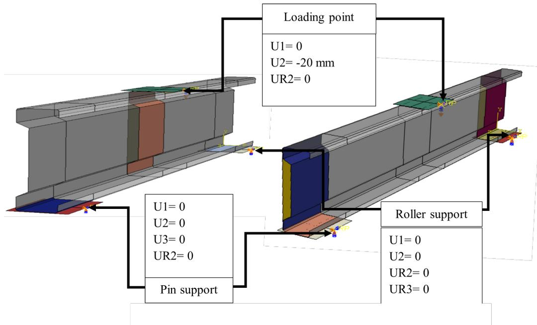
Figure 3: Boundary conditions for EOF and IOF load case
