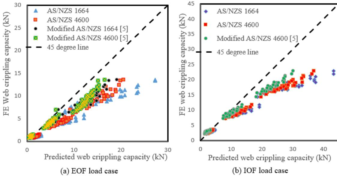
Figure 6: FE web crippling capacity comparison with existing design equations.
