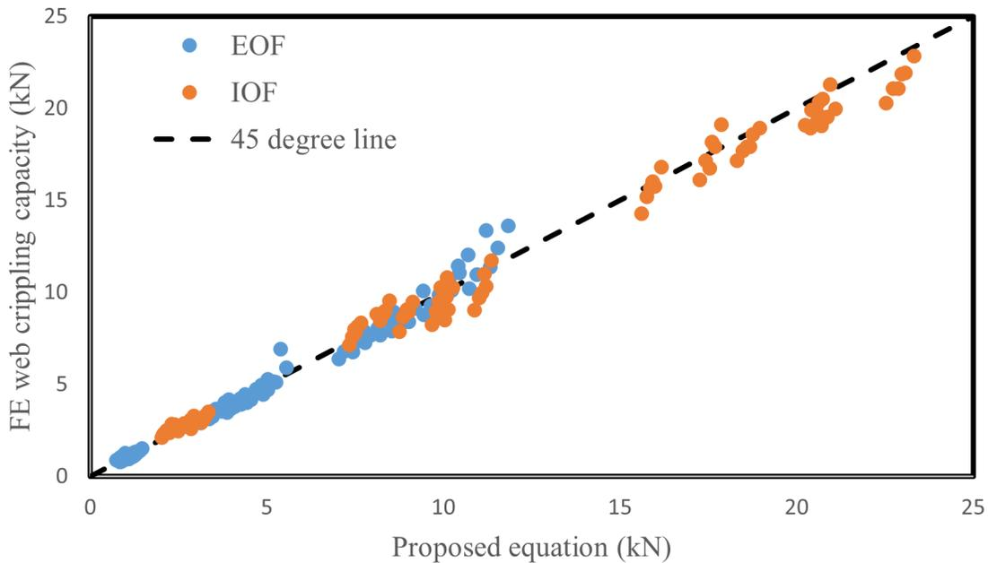
Figure 7: FE web crippling capacity comparison with proposed design modifications.
