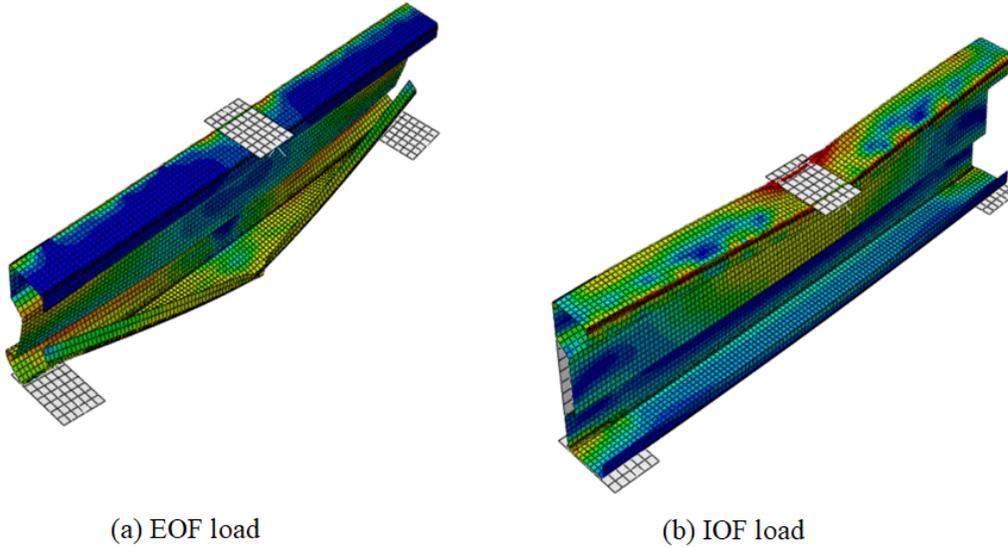
Figure 5: Failure type patterns of aluminium sigma sections under one flange loading conditions.
