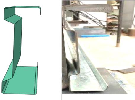
Figure 2: Sigma section profile and numerical model
