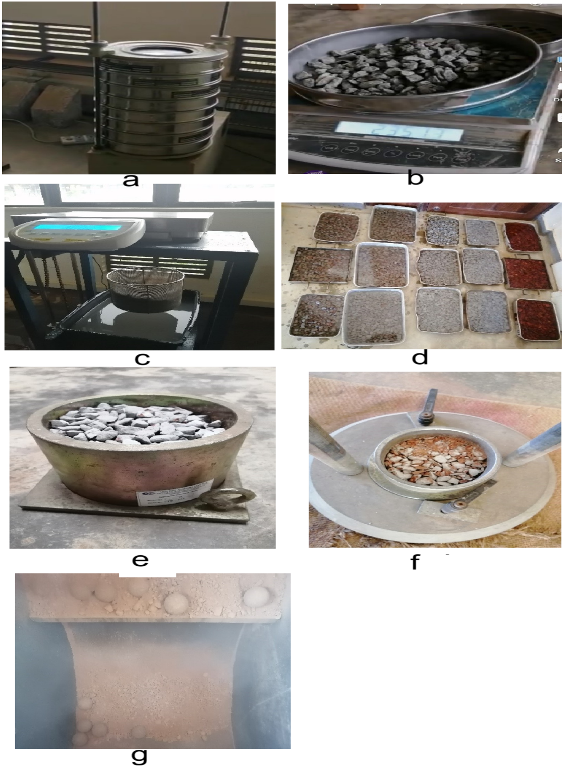
Figure 5: Investigation of aggregate characteristics:(a) Sieve analysis, (b) Bulk density, (c) Specific gravity and water absorption, (d) Moisture content, (e) Aggregate Crushing Value, (f) Aggregate Impact Value, (g) Los Angeles Abrasion Value
